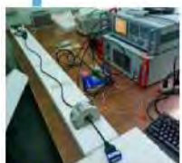
BCI test environment (ISO 11452-4: 2011)
